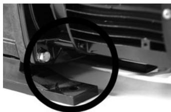
Regularly check the waterproofness! (A leak through a mechanical seal can cause important damages!)
