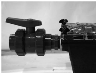
Starting up only with open valves
